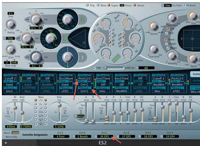
Fig. 1. Logic's ES2, with CC16 (our ribbon/X-axis) set up as Ctrl C, routed to Pitch123 (to control all three oscillators at once). You set range or depth by moving the orange and green triangles.
