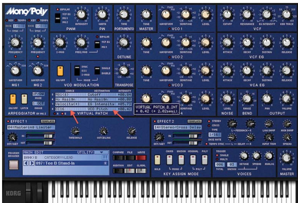
Fig. 2. Korg Mono/Poly, with CC16 routed to VCO Pitch (to control all oscillators at once). Intensity is set to approximately two semitones.
